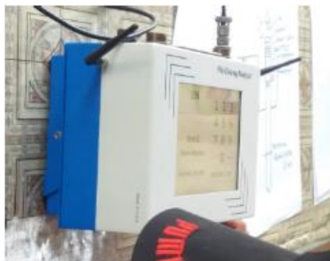
Gambar 1. Alat Pile Driving Analyzer Test
