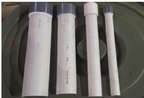
**Gambar 2.** Variasi Diameter Pipa PVC 2inch, 2.5inch, 3inch, dan 4inch Panjang 30 cm
