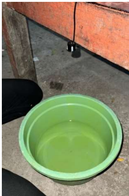
Gambar 6. Pengujian Sensor Ultrasonik Waterproof
