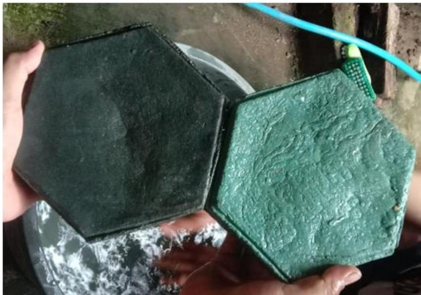
**Gambar 4.** Hasil akhir paving block.
